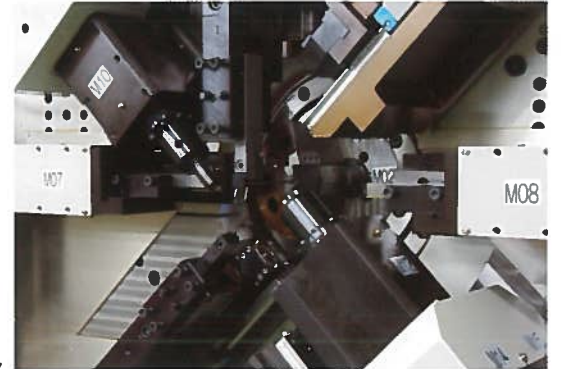
Upper/Lower tables travel 40mm from side to side Quill travels 60mm back-and-forth
